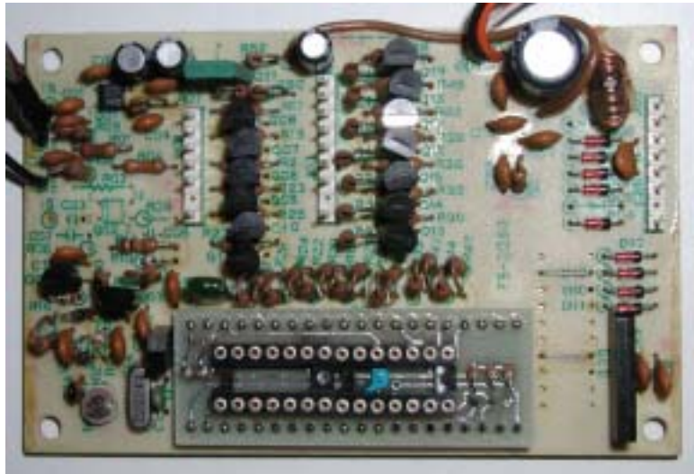
Fig. 8 Completed COUNTER DISPLAY UNIT (w/o PIC16F873)
